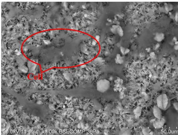
Fig. 4 SEM micrograph of MG63 cells seeded on the \beta -TCP coated Mg for 10 days
